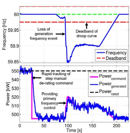
Field test data that shows a single turbine tracking a step change in the de-rating command followed by primary frequency control response to an under-frequency event
