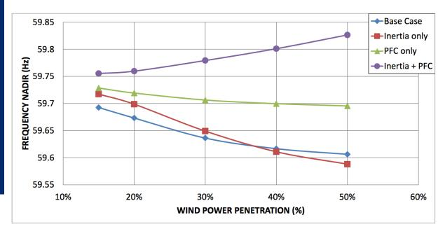
Figure: Impact of wind power controls on frequency nadir
