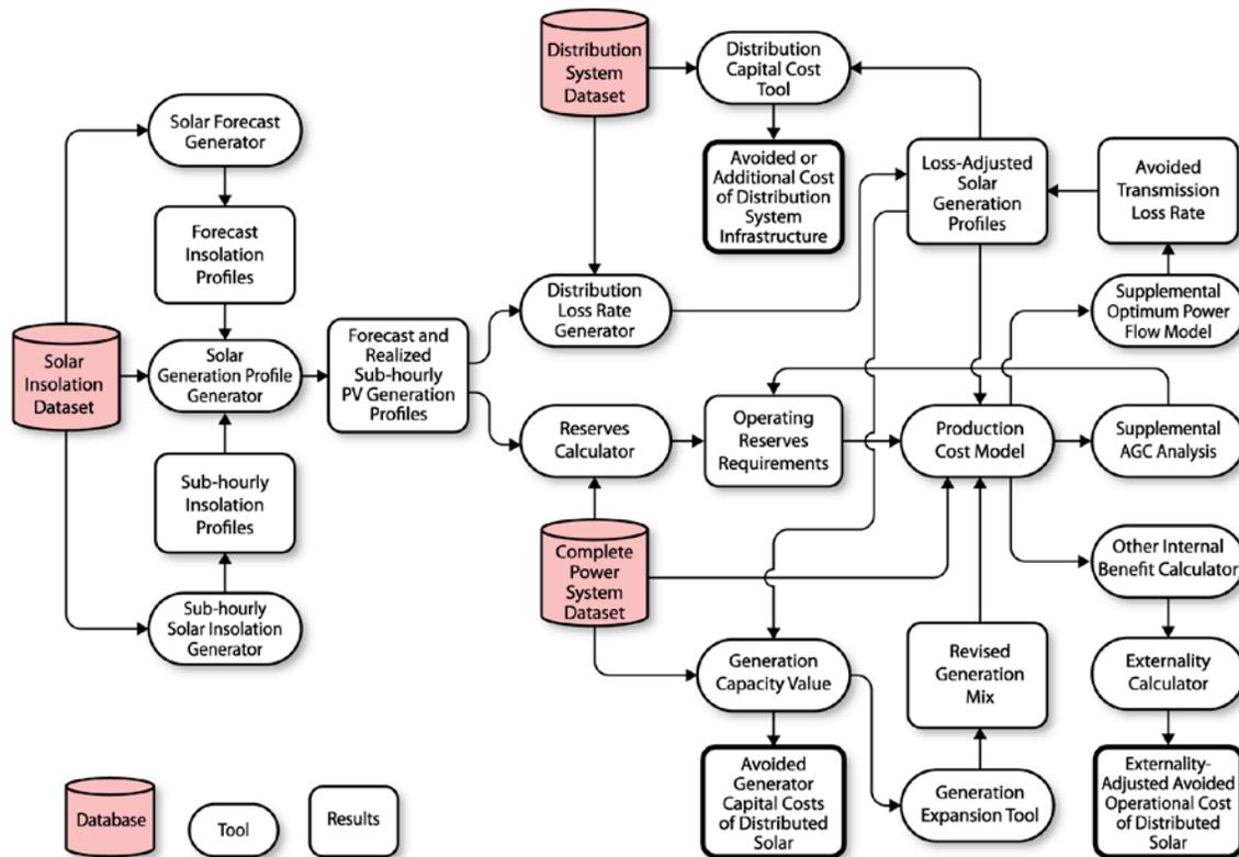
**Figure 6. Possible flow of an integrated DGPV study**
