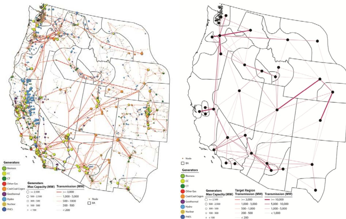
Figure 3. Nodal transmission (left) and zonal transmission (right) representation in WECC<sup>34</sup>
