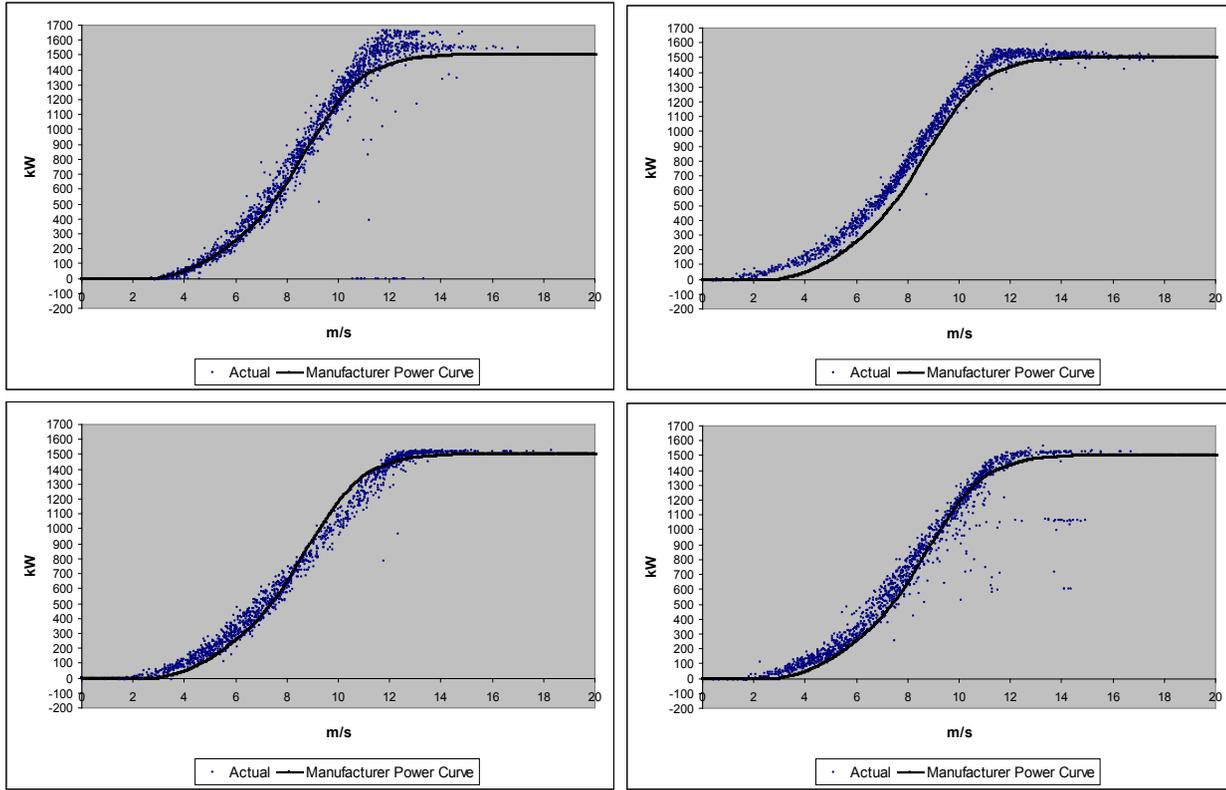
A representative turbine by turbine type by plant was selected for data mining. Wind speed and generation data was averaged over 15-minute intervals. The most predictive equation for current generation was derived from the previous generation and wind speed and the current wind speed. When forecasting, the forecasted wind speed is substituted for the current wind speed in a recursive equation (1a). The previous 15-minute observed power and wind speed initializes the equation (1b).
