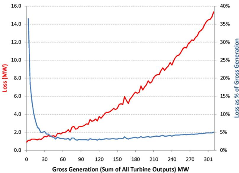
The plant output is the sum of two group outputs minus plant losses with the losses being estimated based on Figure 6.
