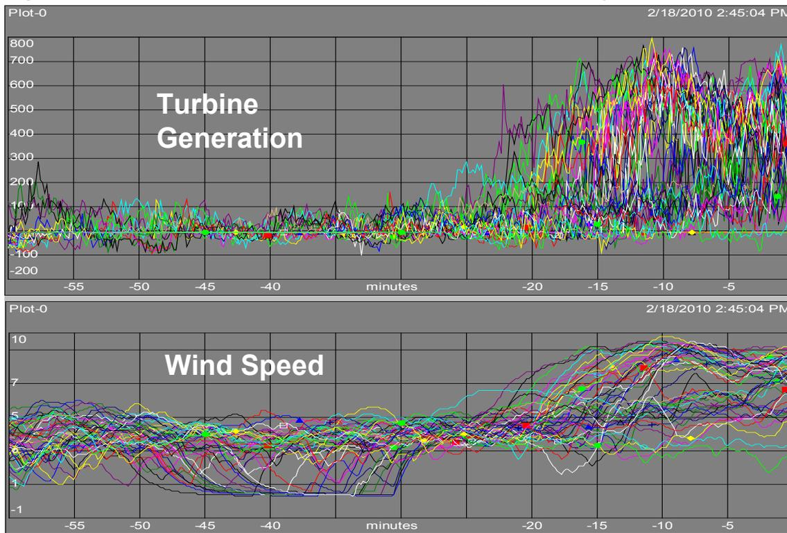
The turbine data are used throughout the wind forecasting system to initialize the weather forecasting cluster, calibrate wind speed forecasts, initialize power conversion, and establish performance metrics.
