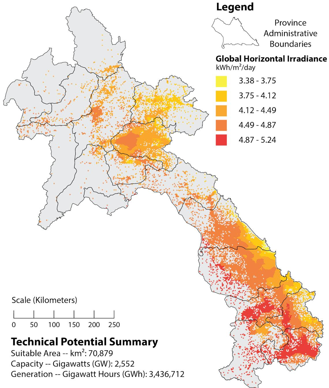
**FIGURE B-2. MAP – SOLAR PV TECHNICAL POTENTIAL: BASE-UXO WITH DEVELOPMENT CONSTRAINED TO AREAS WITH UXO**
